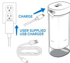
Ensure contacts on BOTH the cable and unit are clean and dry, and the reservoir is emptied and reset (close to the collapsed port) before connecting the charger.
